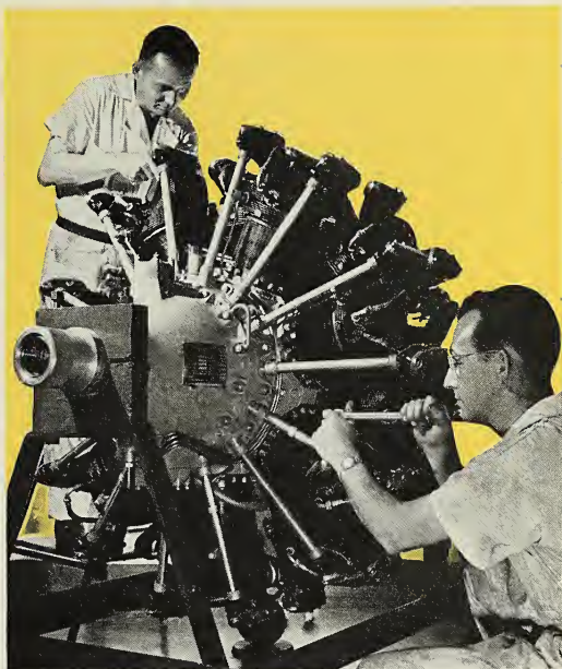
This is an 840 hp, two-row, 14-cylinder, radial air-cooled Italian Fiat engine. It has a geared supercharger and is used to power such planes as the Macchi 200 fighter, the Fiat G-50 fighter, the CR-42 biplane and RS-14 bomber-reconnaissance seaplane.
